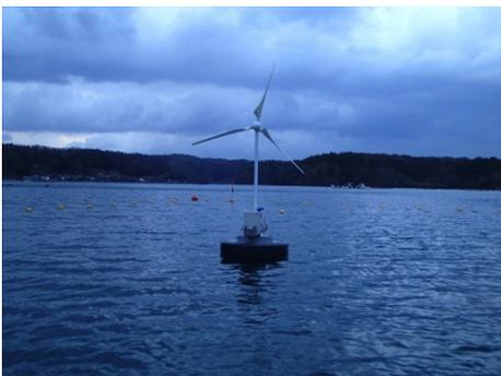
図 2.12: Photo of the FWT model in the real sea test
