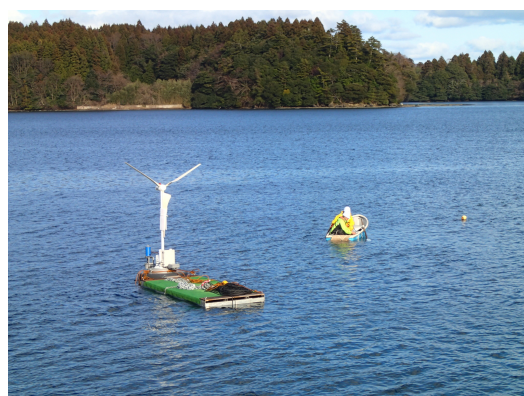
(d) Towing of the wind turbine and other devices on the salvage barge
